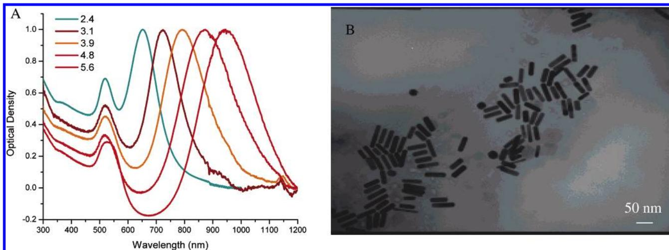
**Figure 1.** (A) Surface plasmon absorption spectra of gold nanorods of different aspect ratios, showing the sensitivity of the strong longitudinal band to the aspect ratios of the nanorods. (B) TEM image of nanorods of aspect ratio of 3.9, the absorption spectrum of which is shown as the orange curve in panel A.
